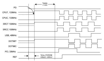
Figure 5. Power-down Deassertion Timing Waveform
