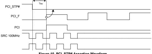
Figure 10. PCI\_STP# Assertion Waveform
