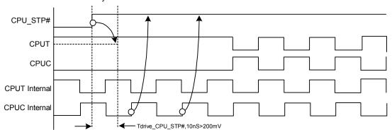
Figure 7. CPU\_STP# Deassertion Waveform
