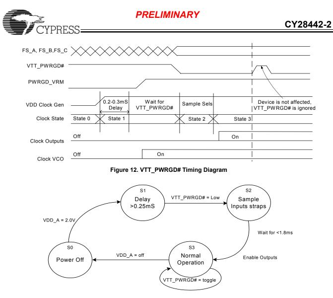
Figure 13. Clock Generator Power-up/Run State Diagram
