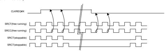
Figure 3. CLK\_REQ#[A:B] Deassertion/Assertion Waveform
