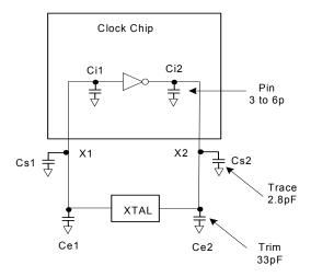
Figure 2. Crystal Loading Example
